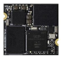
UCM-iMX93L is the very latest generation System on Module from NXP, delivered in an ultra-miniature form factor with energy flex architecture and state-of-the-art security to support energy-efficient edge computing.
